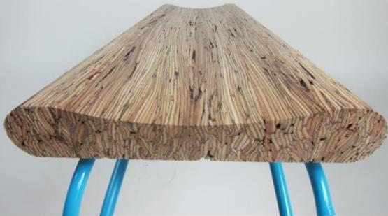
The timber material Lignolit, at the changed production parameters, can be used in the manufacturing of floor panels on the basis of natural wood as a panel-stabilizing element.
